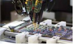
Leading equipment for all kinds of tests e.g. Flying Probe, Boundary Scan, Functional Test.
