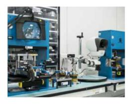
\* Jigs and Tools for bending the electronic components including a Flex machine able to cover several packages and dedicated tools for FPs including QFP 352 and QFP 256.
