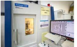
Y. Cougar SMT facility, manufactured by Fein Focus to perform X-RAY inspection both at component and assembly level.
